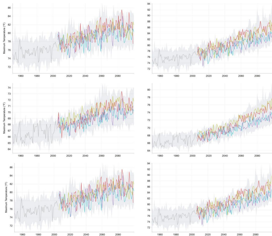
Figure 2. The historical and projected maximum temperatures (°F) in California for the period 1950–2099 for Shasta, Sacramento, and Los Angeles County (top to bottom). Left: projection based on Representative Concentration Pathways, RCP4.5 and right: RCP8.5. Extracted from Cal-Adapt interactive web portal [13].
